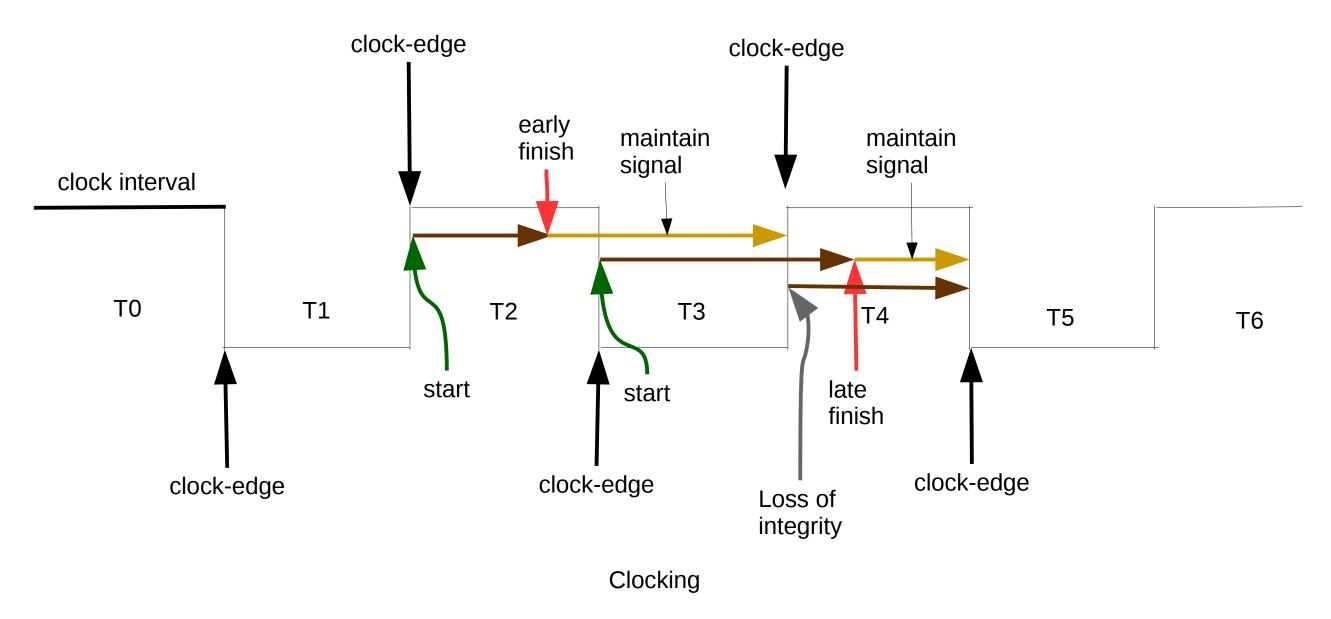
The logic gate takes some time to start, execute, and settle to propagate its signal to the next logic gate. This must be accomplished between clock-edges. Then its output signal is maintained for 1 full clock interval following the clock interval in which is started. Late finishes denote loss of data integrity.
